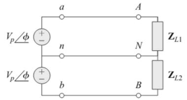
A system in which the ac sources operate at the same frequency but different phases is known as Poly-Phase System.
