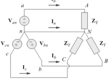
The line-to-line voltages or simply line voltages  $V_{ab}$ ,  $V_{bc}$ ,  $V_{ca}$  can be related as;
