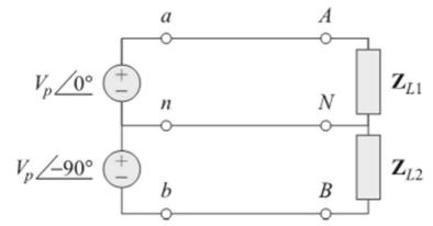
A three-phase four wire system contains three identical sources but different in phase.
