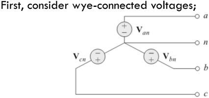
The voltages  $V_{an}$ ,  $V_{bn}$ ,  $V_{cn}$  are respectively between lines a, b, c and the neutral line n.
